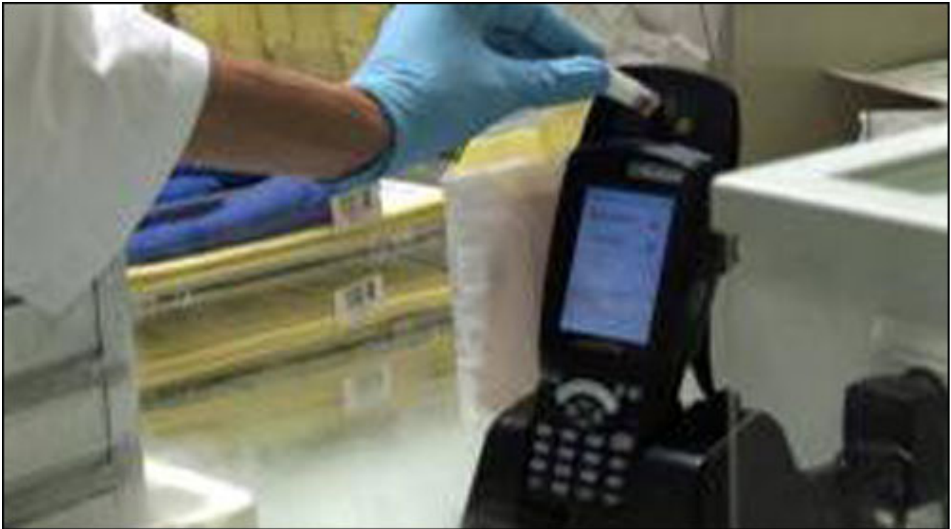
When personnel need to locate particular samples or conduct an inventory of the cryotubes, they can use handheld HF RFID interrogators to read the tags.
