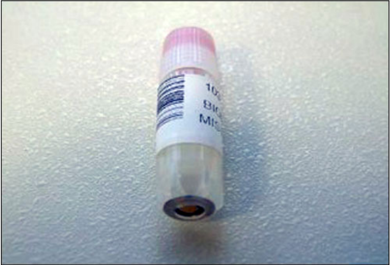
Specimens are placed in individual cryogenic tubes identified with passive HF 13.56 MHz RFID tags.
